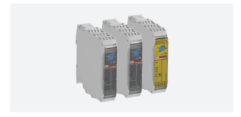
ABB's electronic compact starter packs more functions into less space. The compact unit is just 22.5 mm wide and is suitable for three-phase motor loads up to 3 kW - 400 V AC. Direct-on-line and reversed starter with overload protection and emergency stop versions are available, making the range a perfect fit for high frequent and reliable long life switching of e.g. paper machines, conveyors, pumps, compressors and machine tools.
